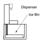
Ice cooled systems have ice bins with ice that is used to cool the product and to fill the cup. It is important that the ice bin be cleaned daily and sanitized according to the manufacturers instructions. Since the ice from the bin is food, the bin must be kept clean.
