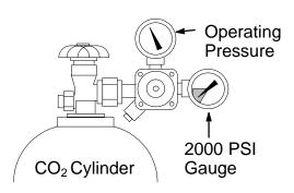
The  $CO_2$  cylinder regulator has a 2000 PSI gauge that indicates the internal pressure in the cylinder. This gauge shows when the cylinder is about to go empty. The gray area at the zero end of the scale indicates that all the liquid  $CO_2$  has been used and only gas remains. This is the ideal time to change the cylinder – before you run out. The cylinder valve must be open or the gauge will not register.
