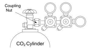
Using a wrench, loosen the coupling nut and remove the regulator from the cylinder. It is normal for a small amount of  ${\rm CO_2}$  gas to escape when removing the regulator.
