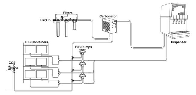
Post-Mix Syrup Bag-in-the-Box containers contain 5 gallons of syrup. When a containers becomes empty it is simple to remove it and replace it with a full container.
