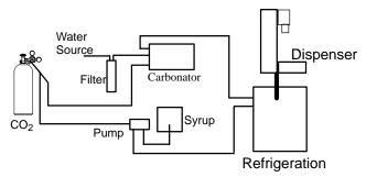
A remote system separates the dispensing valves from the refrigeration system. Carbonated water or water bath water is circulated between the refrigeration unit and the dispensing valves to insure that a cold product will be dispensed.
