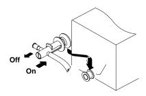
On a new Bag-in-Box container pull out the bag fitting and lock it in place with the box tab.
