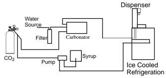
With an ice-cooled system the refrigeration type is the main difference. Here the refrigeration consists of a bin which holds ice and has a cold plate in the bottom, through which the syrup and water is cooled for your post-mix drink.
