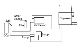
The post-mix countertop system is a common setup. Here the relationship of the dispenser, carbonator, water, syrup and CO<sub>2</sub> are shown.
