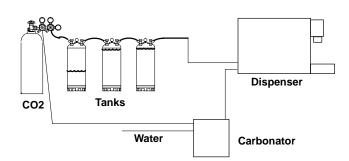
If you have three tanks on your fastest moving flavor, the tank closest to the CO2 supply will go empty first, then the middle tank and then the tank closest to the dispenser. When removing empty tanks always remove the empty tank, "C" in this example, move the partial tank, "B", so it is closest to the CO2 supply. Next in line should be the full tank, "A" and then install the new tank in the position closest to the dispenser.
