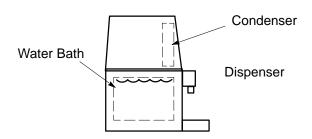
Electrically operated refrigeration systems rely on a clean condenser to ensure maximum ice production and product cooling. If the condenser is dirty, it can be cleaned with a soft brush or a vacuum. Also check the water bath level. If the water level is not within 1 inch of the overflow, the water bath must be filled until the water overflows the water bath and runs into the drip tray.
