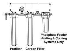
Many filter systems use a gauge at the filter outlet to indicate the pressure at the outlet. As the filter becomes plugged, the pressure will drop at the outlet.
