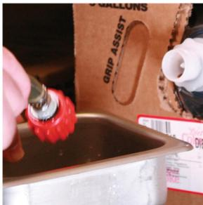
**Step 5.** Soak connectors in chlorine based sanitizer solution for 1 minute.
