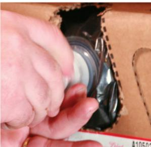
**Step 4.** Pull the bag connector through the opening and remove the plastic dust cap.
