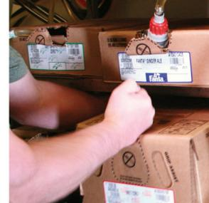
**Step 3.** Open the flap of the new box by hitting it sharply with your palm. **DO NOT** use a sharp instrument.
