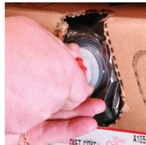
**Step 6.** Reconnect to the correct Bag-in-Box. Tighten until the connectors are fully engaged.
